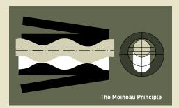
The progressing cavity pump itself is based on the Moineau principle. A rotor turns within a stator, creating a sequence of sealed chambers. The precision-cast and polished stainless steel rotor moves wastewater through these chambers at a nearly constant flow, over a wide range of conditions – from negative to abnormally high heads. Turning at just 1,725 rpm, the one-horsepower motor can pump fluid through more than two miles of small-diameter piping or elevation changes of over 185 feet.
